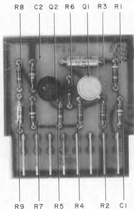
Figure 5-35. Type 7312 Video Amplifier (A9), Location of Components
